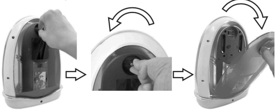
**2.** Remove the battery cover at the bottom of the clock.
